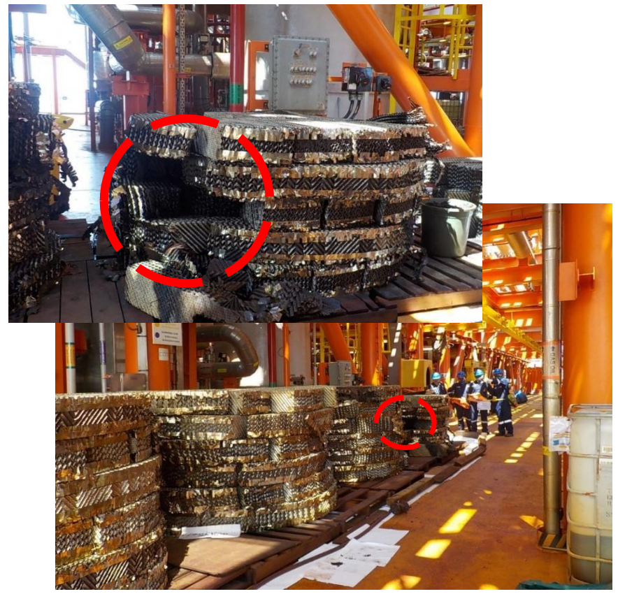
The data is confirmed, Bed packed condition after the column is dismantled, there are denser and cavity area on the bed packed due to operation.
